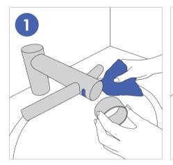
Wipe sensors using a soft cloth and non-abrasive cleaner then place cleaning cap over sensors to prevent air and water from being activated.
