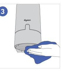
REGULARLY clean air inlets on base of motor bucket (under sink). Ensure plughole in sink is free from blockages so water can drain freely.
